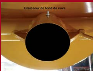
Greasing of bottom of drum
